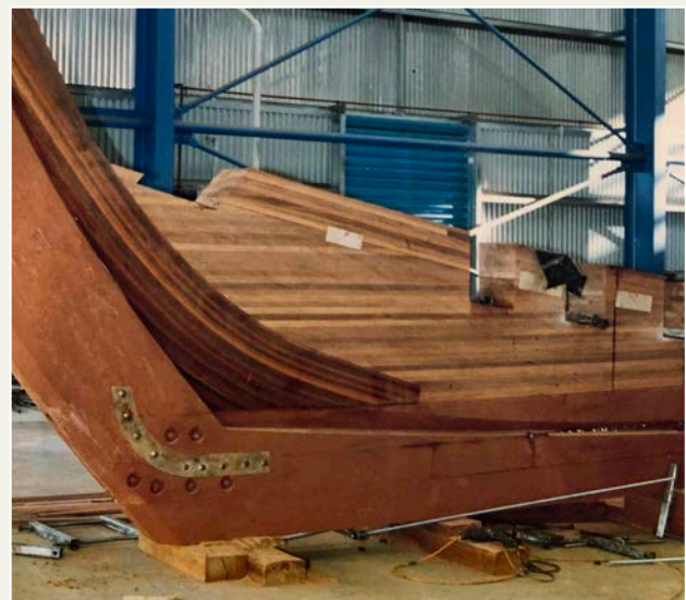
Figure 25. Endeavour replica stem and keel after being joined, showing the scarph, bolt pattern and modified horseshoe plate (HM Bark Endeavour Foundation, Australian National Maritime Museum Collection).
